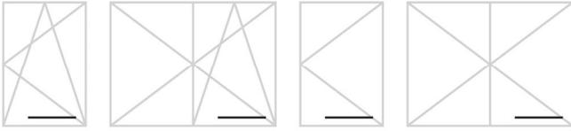
**Figure 2:** Preferred installation position of a casement stopper
