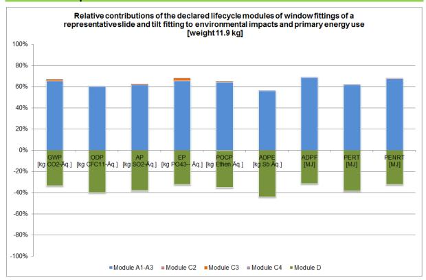
The largest contribution to **Global Warming Potential (GWP, 100 years)** comes from preliminary product provision (87%) - mainly from the manufacture of continuous aluminium casting and the silicone seals. 13% of global warming gas emissions are caused by the manufacturing process itself. These are mainly attributable to electricity requirements. A total of 51% of all GWP emissions are credited; the dominant contribution comes from recycling the aluminium (72%).
